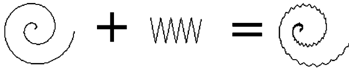
Figure 8. The result of adding two trajectories to produce a compound trajectory
